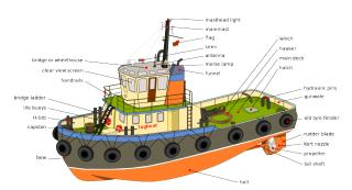
"Tugboat diagram" by Al2 with minor modification s by Lycaon – Own work. Licensed under CC BY-SA 3.0 via Commons.
